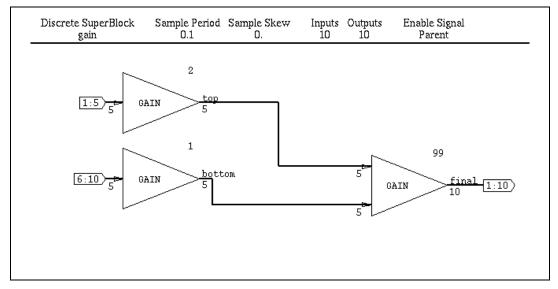
Figure 6-3. Multiple Array Mode
